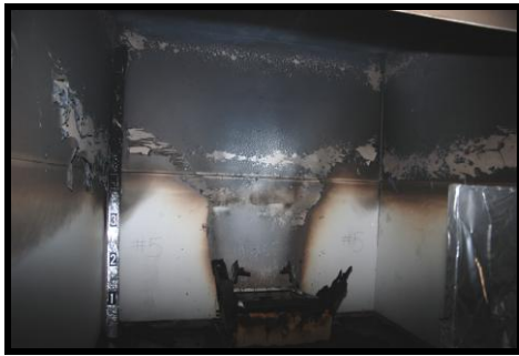
Figure 10: Chair 5 30" Header - Actual Damage (left); Calcination Measurements (center); Thermocouple Data (right)
