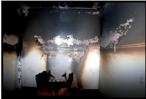
Figure 11: Chair 6 30" Header - Actual Damage (left); Calcination Measurements (center); Thermocouple Data (right)
