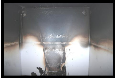
Figure 7: Chair 2 18" Header - Actual Damage (left); Calcination Measurements (center); Thermocouple Data (right)
