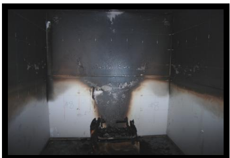
Figure 13: Chair 8 42" Header - Actual Damage (left); Calcination Measurements (center); Thermocouple Data (right)
